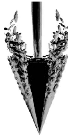
(b) Instantaneous iso-surfaces of vorticity colored by the span-wise component of vorticity of a 70° delta wing. From: Morton (2004)
