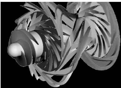
(e) Computer model of the liquid hydrogen pump of the VULCAIN engine of the European launcher ARIANE 5.
